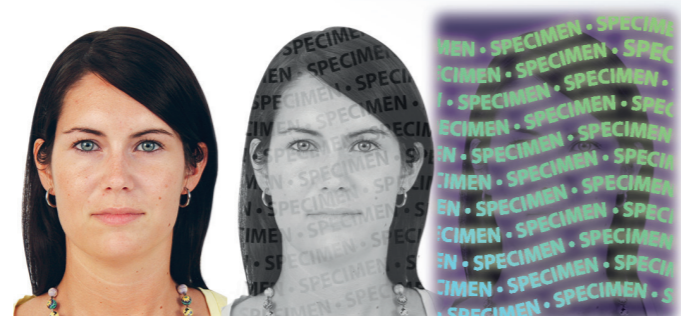
IMAGE UNDER DAY LIGHT IMAGE UNDER INFRARED LIGHT VISUALIZATION OF DTLI UNDER UV LIGHT
