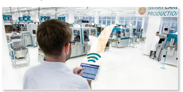
MB PalaMax®, Mühlbauer's Smart Factory solution, is developed for card, tag or booklet productions, personalization factories and semiconductor backend shop floors. Consisting of an NOSQL database, it is designed to set and collect process data to monitor and improve the efficiency of production and personalization. The collected process data is stored in big data sets for later processing, visualization and statistical analysis.
